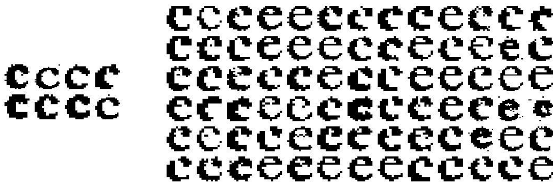
Figure 7: Images misclassified when 60,000 prototypes were used to derive a decision tree (out of the 100,000 tested, shown normalized). On the left: samples of ‘c’s; right: samples of ‘e’s.
