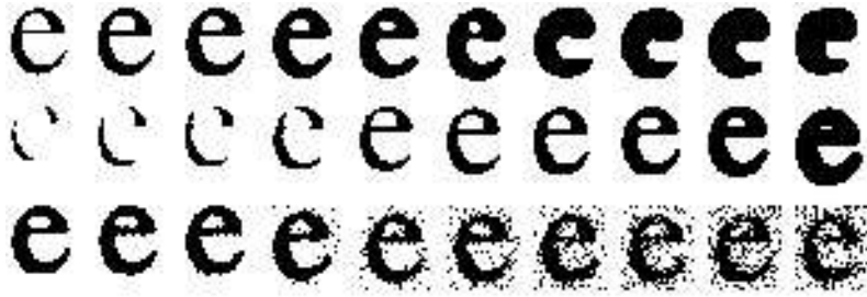
Figure 1: Effects of blurring, thresholding, and pixel sensitivity. Images are created with blur varying from 0.0 to 3.6 by 0.4 (top row); thrs varying from 0.9 to 0.0 by -0.1 (middle row); and sens varying from 0.0 to 0.9 by 0.1 (bottom row).
