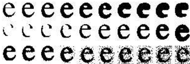
Figure 7: Effects of blurring, thresholding, and pixel sensitivity. Images are created with blur varying from 0.0 to 3.6 by 0.4 (top row); thrs varying from 0.9 to 0.0 by -0.1 (middle row); and sens varying from 0.0 to 0.9 by 0.1 (bottom row).
