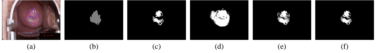
Fig. 1. Training multiple SVM classifiers in the ensemble for AW segmentation. (a) Original image with AW boundary markings by multiple medical experts; (b) The ground truth map computed by MOSES; (c) AW segmentation by SVM classifier 1 ( p = 0.576, q = 0.988 ); (d) AW by classifier 2 ( p = 0.954, q = 0.632 ); (e) AW by classifier 3 ( p = 0.776709, q = 0.967 ); (f) AW by classifier 4 ( p = 0.655, q = 0.990 ).
