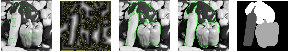
Fig. 11. Boundary finding in the pepper image. (a) Original image, with initial models drawn on top. (b) The shape image derived from the edge map. (c) Intermediate result showing the models after 10 iterations. (d) Final converged models after 14 iterations. (e) The three pepper segments enclosed by the three converged models.
