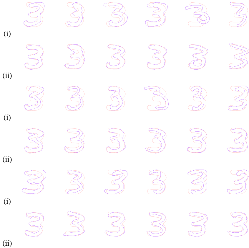
FIGURE 3. Global registration using the affine transformation model. (i) initial pose (ii) affine-invariant registration (the same target contour is used).
