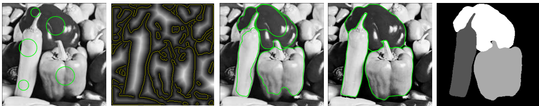
Figure 3.14: Boundary finding in the pepper image. (a) Original image, with initial models drawn on top. (b) The shape image derived from the edge map. (c) Intermediate result showing the models after 10 iterations. (d) Final converged models after 14 iterations. (e) The three pepper segments enclosed by the three converged models.
