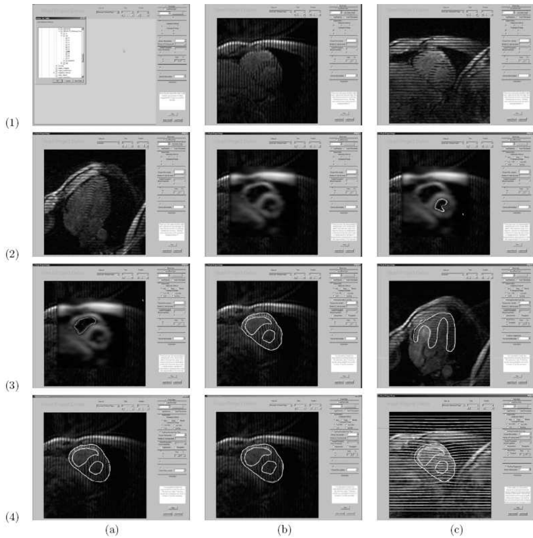
Figure 6.5: Screen snapshots of the 4D tagged MR analysis system. (1-a) reading in the SA and LA volumes. (1-b,1-c,2-a) examining the data sets. (2-b) de-tagged image at the center time. (2-c,3-a) Metamorphs segmentation on the de-tagged images. (3-b,3-c) segmentation results at the center time. The papillary muscle is excluded from the myocardium by manual interaction. (4-a,4-b) temporal propagation of the segmented contours. (4-c) tagging lines tracking.
