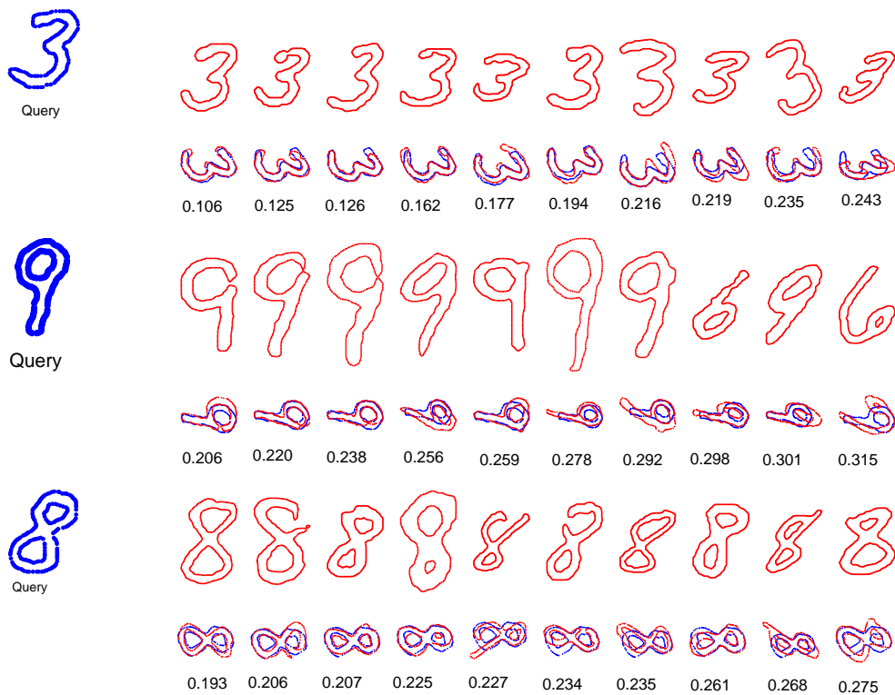
Figure 9: Recognition and Matching results on a set of 200 handwritten digit shapes. The left-most blue shapes are the query shapes, for each query shape, we show its top 10 closest test shapes in the first row, and show the test shapes (red) and the query shape (blue) matched together in the second row, the distance between each test shape and the query shape is also shown. In the top ten matches for digit 9, some digit 6 shapes appear because the two shapes are similar after rotation and scaling.
