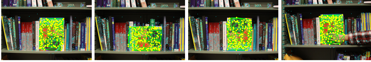
Figure 2. Matching the Spectrum magazine (Fig. 1(a)) in scene images with cluttered background. (From left to right) the magazine is not rotated, rotated by 90 degrees, rotated by 180 degrees, and occluded by a hand. Unmatched scene feature points are marked in light blue.
