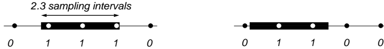
Figure 3: Sampling a black stroke 2.3 sampling-intervals long may yield a bitmap of 3 or 2 black pixels.
