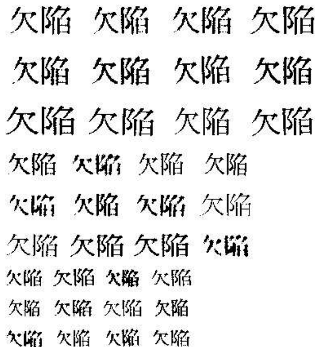
Figure 1: Thirty-six images of the Japanese word ‘kekkan’ (defect), from the JTeX Mincho typeface, illustrating the range of image defects generated pseudo-randomly by a model discussed in the text. There are twelve samples for each of three point sizes (10, 8, and 6), at a spatial sampling rate of 300 pixels/inch. The images are magnified in order to make the spatial sampling rate visible.
