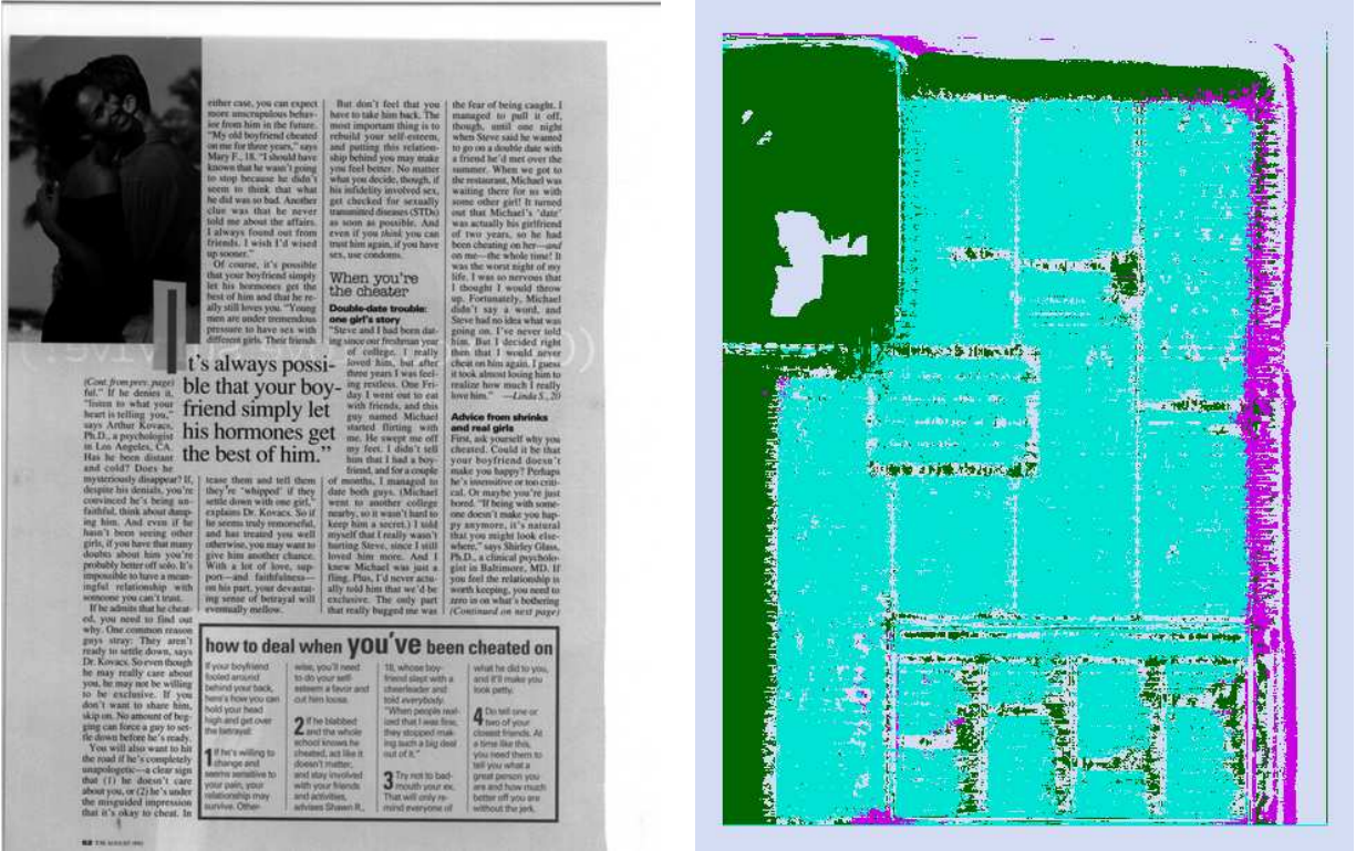
Figure 1. A bilevel document image (on the left) and its per-pixel classification (on the right). Dark green indicates the photo (PH) content class (concentrated along the left edge and upper left corner), light blue indicates machine print text (MP) (most of the center of the page), magenta indicates handwriting (HW) (along the right margin and scattered), and light gray indicates unclassifiable (JK) (the outermost margins). Although the per-pixel classification correct rate is only 77%, the principal regions and their identities are clearly indicated and it may be possible to refine them reliably in post-processing stages.
