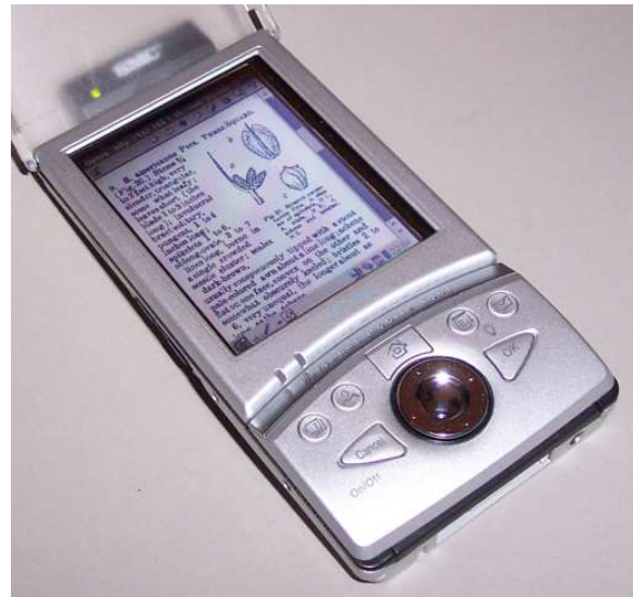
Figure 5. On this PDA a passage of text-image from Jepson’s Flora has been reflowed onto the small display, i.e. the images of its words have been moved about and broken into shorter text-lines in order to fit legibly. No OCR was attempted; thus no recognition errors are visible. The original appearance of the specialized and meaningful typography, reading order, and the proximity of line-art Figures to their first mention in the text, are preserved.
