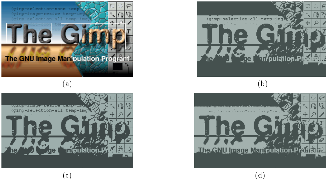
Figure 2. (a) Test image “The Gimp” with text boxes marked, (b) Binarization with k -means, (c) Binarization with the ACR benchmark, 19 (d) Binarization with Algorithm 1.
