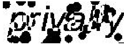
Fig. 6. Example of a BaffleText challenge: a nonsense (but English-like) word was generated pseudorandomly, the word (as a whole) was typeset using a randomly chosen typeface, an mask was generated, and the word image was damaged using the mask.
