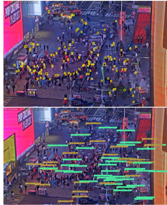
Figure 2: A real-world webcam image of New York City's Times Square reveals the complicated nature of the problem. Top: faces detected using RetinaFace [5]; Bottom: face mask detection using Mask-RCNN [7].
