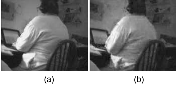
Fig. 1. Result of decoding ka15p using floating point with oddification (IEEE-1180) for (a) Frame 46 does not exhibit IDCT mismatch because it is an I frame; (b) Frame 45 does exhibit IDCT mismatch because it is the result of a long string of P frames.
