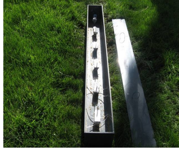
(b) PVC box with sensors before soil filling
