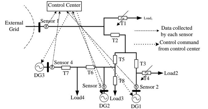
Fig. 1. Microgrid with centralized control.
