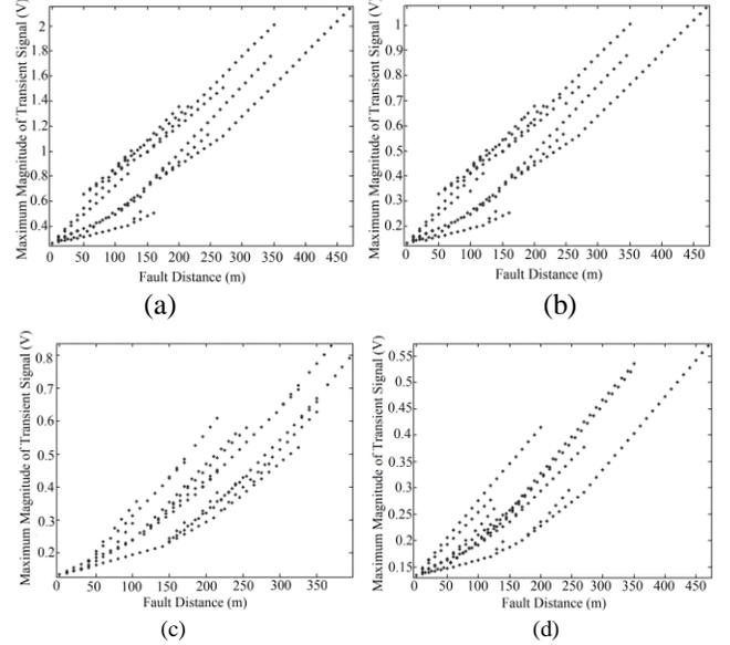
Fig. 9. The relation between transient signal magnitude and fault distance: (a) a 220v microgrid with topology A and parameter set A (Case 1); (b) a 110v microgrid with topology A and parameter set A (Case 2); (c) a 110v microgrid with topology B and parameter set A (Case 3); (d) a 110v microgrid with topology A and parameter set B (Case 4).
