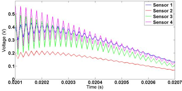
Fig. 3. Zoom-in view of transient voltage signals caused by a short circuit at T4 in a microgrid depicted as Fig. 1 during fault time.
