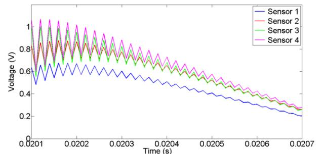
Fig. 2. Zoom-in view of transient voltage signals caused by a short circuit at T1 in a microgrid depicted as Fig. 1 during fault time.
