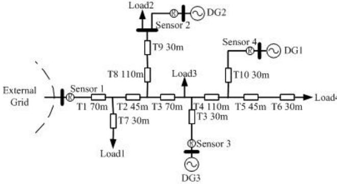
Fig. 8. Simulation topology, microgrid B.
