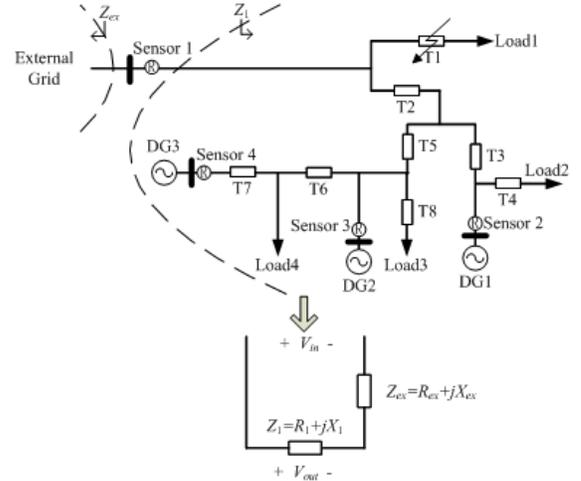
Fig. 4. Equivalent circuit of a short circuit.
