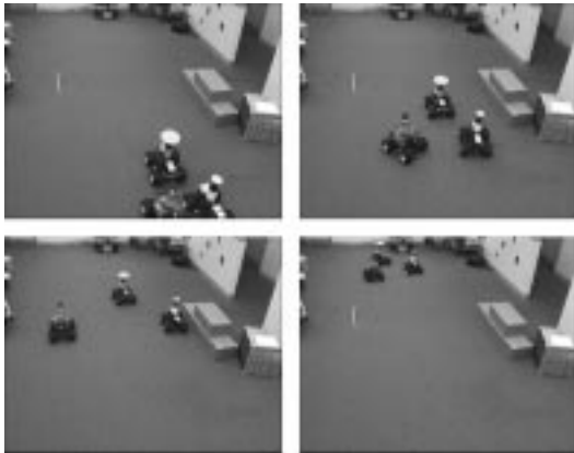
Figure 9: Trajectory for two pursuer robots tracking a moving target robot in a cluttered workspace. The left pursuer adapts its trajectory to the right pursuer’s mobility constraints.
