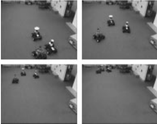
Figure 7: Trajectory for two pursuer robots tracking a moving target robot in an obstacle-free environment.
