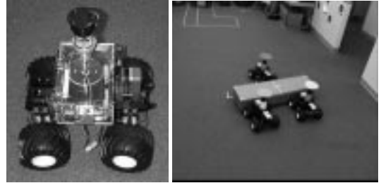
Figure 1: A single Clodbuster robot (left) and the team performing a distributed manipulation task.
