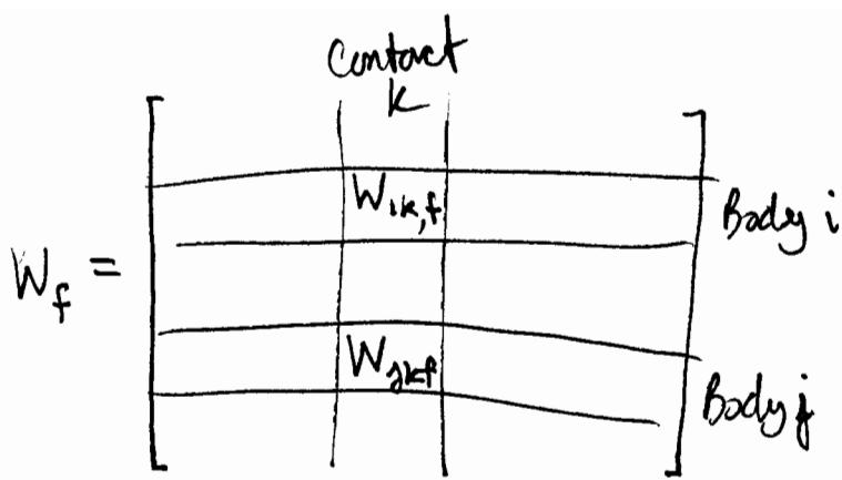
$$W_{ik,f} = \begin{bmatrix} \hat{d}_{ik,1} & \dots & \hat{d}_{ik,n_f} \\ r_{ik} \times \hat{d}_{ik,1} & \dots & r_{ik} \times \hat{d}_{ik,n_f} \end{bmatrix}$$
