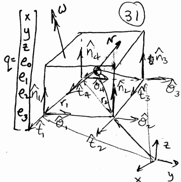
$${}^N W_n = \begin{bmatrix} {}^N \hat{n}_1 & \dots & {}^N \hat{n}_4 \\ {}^N r_1 \times \hat{n}_1 & \dots & {}^N r_4 \times \hat{n}_4 \end{bmatrix}$$
