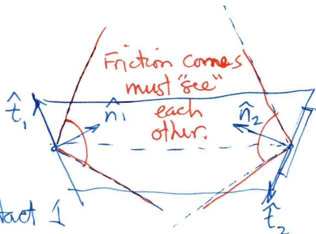
Keeping contact 1 fixed, determine how far contact 2 can be slid up edge and keep contact 1 in its friction cone.
