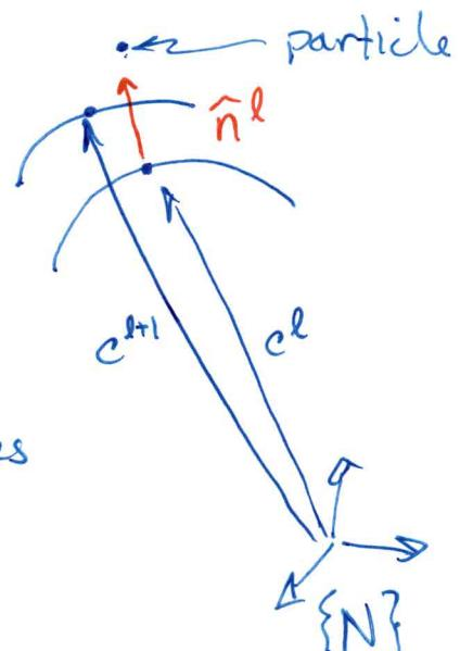
Note: when particle is replaced by a body of finite extent,  $\hat{n}^l$  will be replaced by  $G_n^T = \begin{bmatrix} \hat{n}^l & (r \times \hat{n})^T \\ \vdots & \vdots \end{bmatrix}$ .
