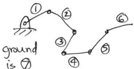
$$\begin{aligned} \cdot 7 \text{ bodies} &\Rightarrow 42 \text{ dof} \\ 1 \text{ is fixed} &\Rightarrow 6 \text{ constrs} \\ 6 \text{ jnts remove} \\ 5 \text{ dof's each} &\Rightarrow 30 \text{ constrs} \\ \hline &\doteq 6 \text{ dof's} \end{aligned}$$
