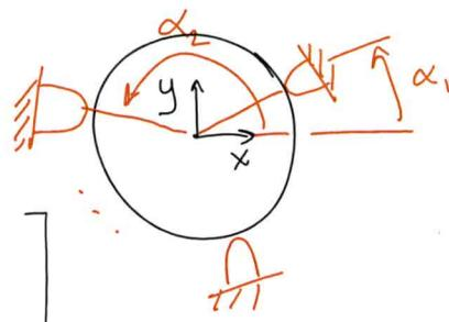
$$G_n = \begin{bmatrix} -\cos(\alpha_1) & -\cos(\alpha_2) & \dots \\ -\sin(\alpha_1) & -\sin(\alpha_2) & \dots \\ 0 & 0 & \dots \end{bmatrix}$$
