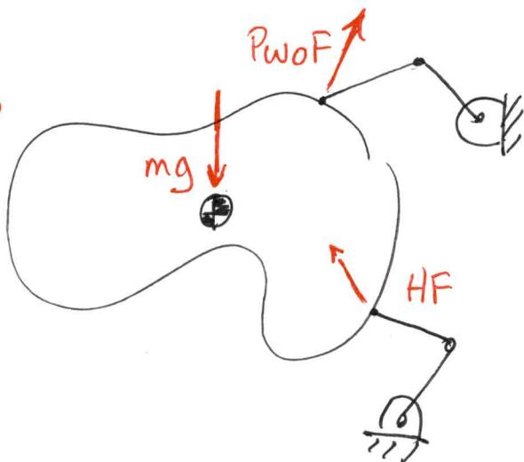
However, for the grasp to be sustained, the force applied to object by PwoF is pulling, but frictionless contacts can't pull.
