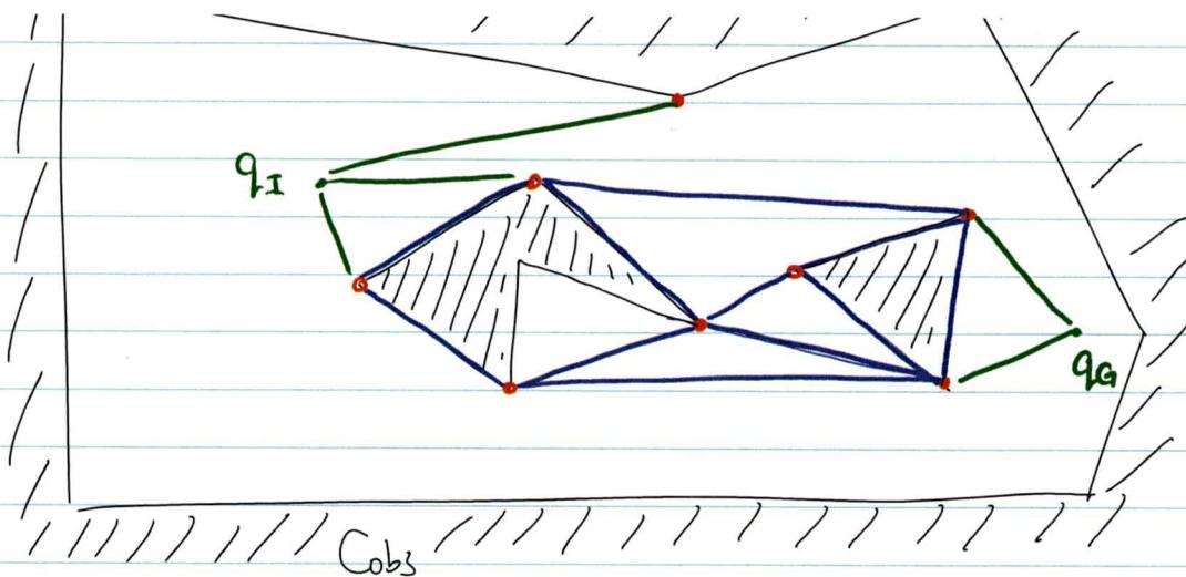
To solve query, insert  $q_I, q_G$ , then create edges from  $q_I \& q_G$  to every visible vertex (see above green links).
