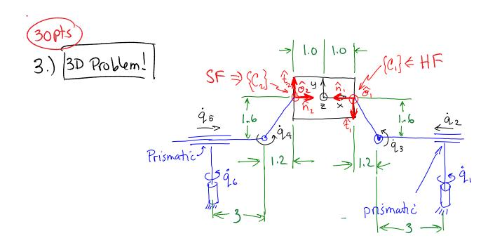
Contact 1 (on right) is a hard finger contact. Contact 2 (on left) is a soft finger contact.
