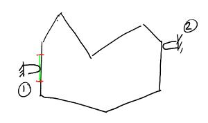
perfectly accurate. Sketch the region of finger @ placements that would yield frictional form closure for every placement of finger @ inside the region shown.
