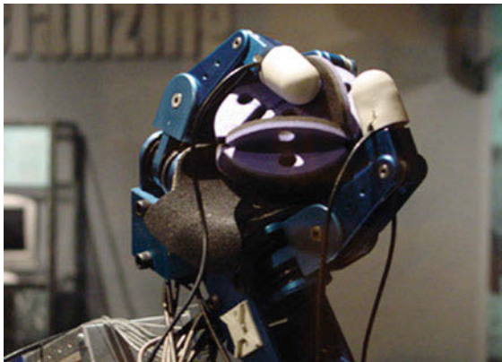
Fig. 38.1 The Salisbury Hand grasping an object
