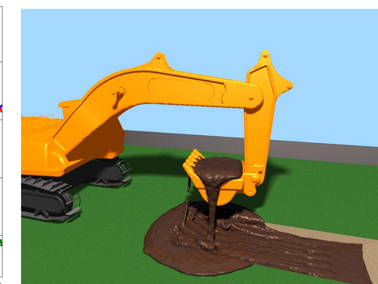
Fig.11 Fluid-Solid Simulation Of Highly Viscous Material Being Scooped By Digger
