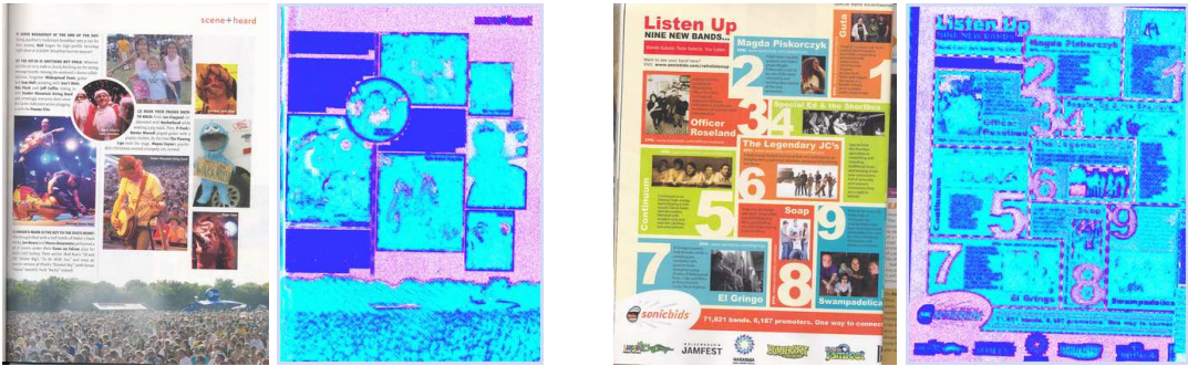
Figure 13. The page on the left illustrates success on a difficult case where the blank region that forms the background of most of the page bleeds imperceptibly into a photograph at the bottom. The page on the right illustrates an unusually complex nonrectilinear layout: when this is studied closely, it reveals many cases of successful discrimination between machine print and photographs on small irregularly shaped regions. Per-pixel accuracies: left 69.3%, right 35.0%.
