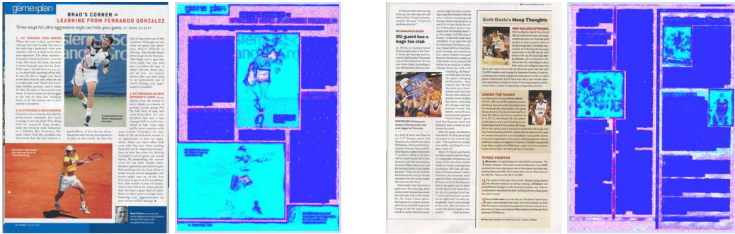
Figure 14. The magazine page image on the left is remarkably well segmented: almost all text, including text embedded within photographs, is correctly labeled. The page on the right illustrates success on related, challenging cases: text overprinted on regions of arbitrary solid color. Per-pixel accuracies: left 70.9%, right 73.8%.
