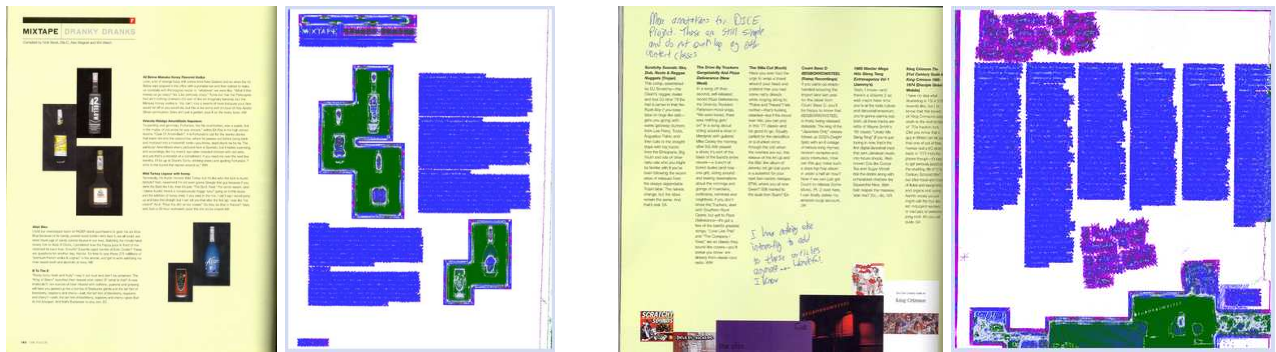
Figure 8. Test page images containing relatively simple magazine article layout. The first image contains blank (shown as white), machine print (blue), and photograph (green) content and the second also contains handwriting annotations (pink). In the first image 86.72% of the pixels were correctly classified and 70.4% in the second. We subjectively rank the segmentation quality as good except perhaps for a fraction—less than 20%—of the photograph regions.
